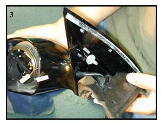
Carefully peel back the foam insulation on the mirror housing sail.
